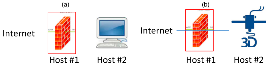
Figure B.1. (Color online) Network Model for Game: (a) PC Version, (b) Equivalent Manufacturing Version
